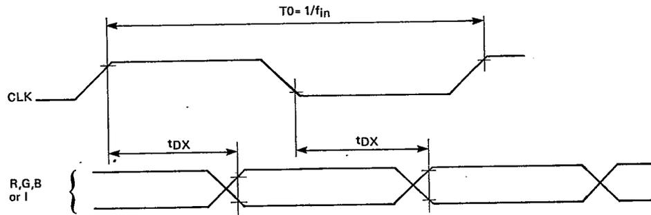
FIGURE 3 - R, G, B and I TIMING (VIN)
