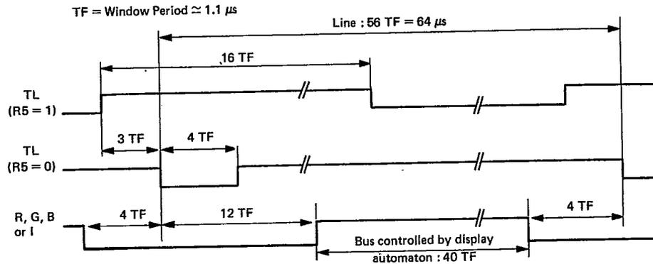
262 line periods (if  $R6 = 0$ ) or 312 line periods (if  $R6 = 1$ ) make a frame period. The TT output is at frame period (60 Hz/50 Hz) and is low during 2 lines. SYT input resets the line count inside the frame : this input is triggered, then sampled when the 12th window of each line occurs. When the sample transits from 1 to 0, the line count will be reset on the next TL.
