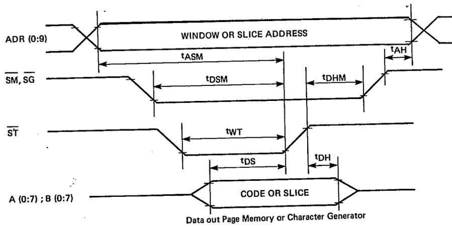
FIGURE 6 - INTERNAL BUS - FROM PAGE MEMORY OR CHARACTER GENERATOR TO MAIL BOX TRANSFER CYCLES (R/Wi= 1)
